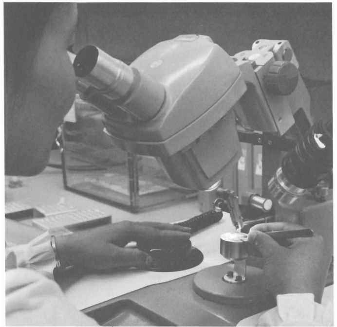
Using gossamer-thin aluminum wire, microscopic connections are made by ultrasonically joining points on an IC chip to the frame. At the controls is F&T's Frances Hartman-Kok.
