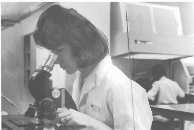
Production and testing of ICs require microscopic techniques. At left, masking and alignment machine operated by Ilona Lehel is visible in background, while Sonia Whitelaw, foreground, inspects a stage in wafer manufacturing. Above is multiple probe, with which operator can simultaneously and automatically test each chip while in wafer form.
