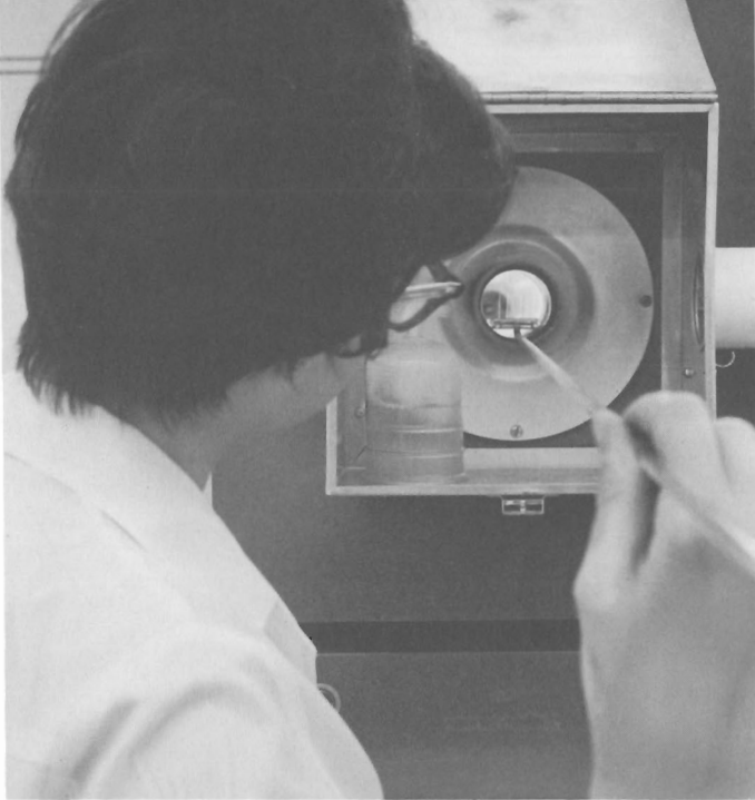
Sharon Martin inserts a "boat" of IC wafers into furnace that treats them at high temperature, one of several major steps in creating finished chips on surface of a silicon wafer.
